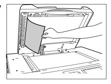
Open the exit-side cover and remove any misfed originals.
